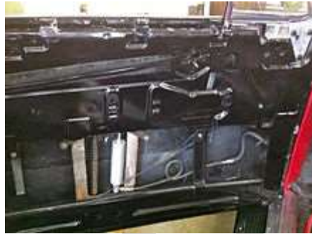
Inside drivers door showing hydraulic cylinder for power window
