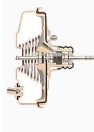
Brake off - both sides of the diaphragm are under vacuum.
