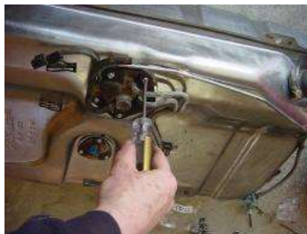
Electric Fuel Pump Replacement
