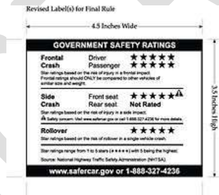
Consumer information label for a vehicle with at least one US NCAP star rating
